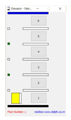
The system may ask an elevator to go up, go down or stop by a panel. The system may ask the elevator to open its door. The system will receive a notification when the door is closed. This simulates the activity of letting people on and off at each floor. The door closes automatically after a predefined amount of time. The touch panel above also shows position (up and down) and the waiting people of the elevator at real time!
